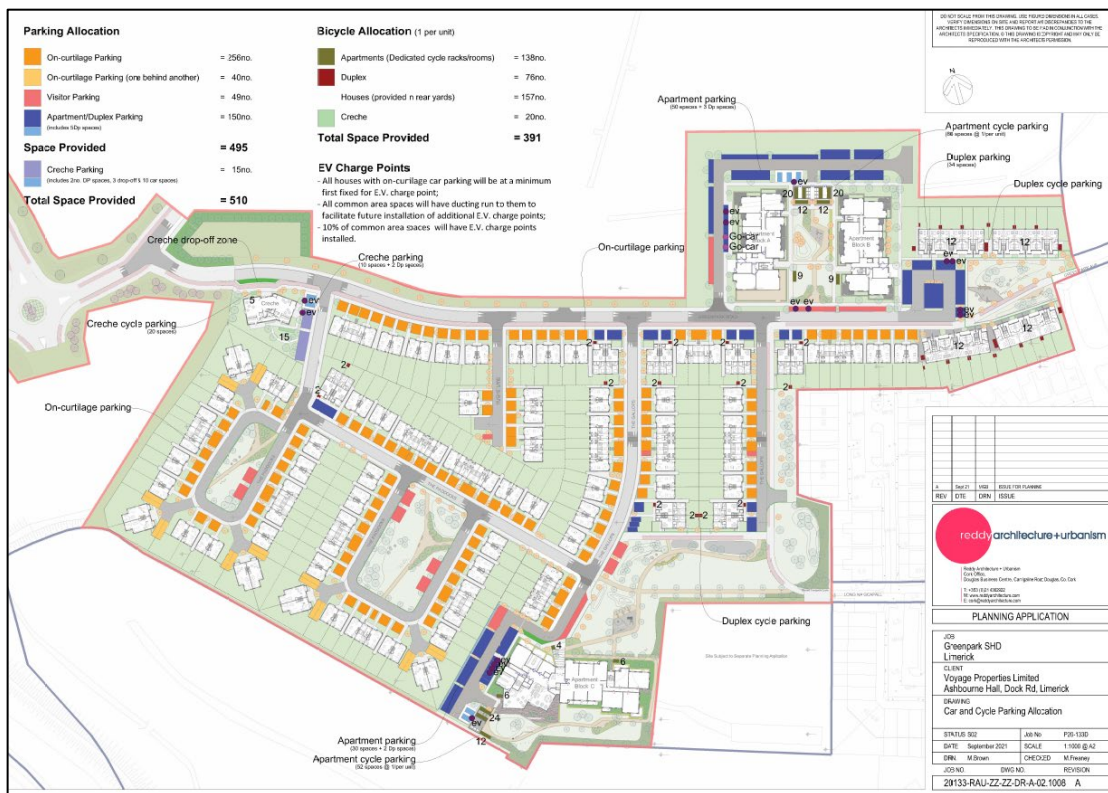
Figure 5.7: Extract from Reddy Architecture + Urbanism’s Dwg. No. ZZ-ZZ-DR-A-02.1008 Rev A showing the car and cycle parking allocation across the site.
